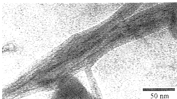
Figure 3. A TEM image of an organogel fiber, mol ratio of 1 is 10%, stained by sodium phosphotungstate.
